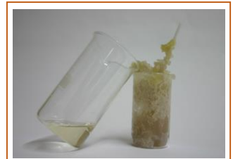
On the right: a resin with 38% micro-filler yields a fissured mass. On the left: the same resin with 40% nano-filler remains a liquid.
