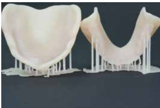
Try-ins made from V-Print Try-In incl. support structures.
