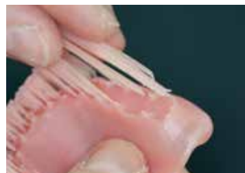
Rapid removal of support structures (design possible with SolFlex 3D printers)
