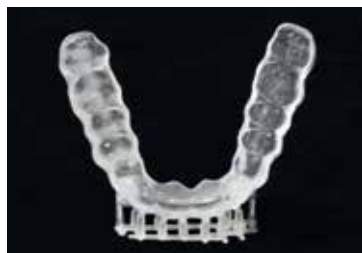
Splint with support structures
