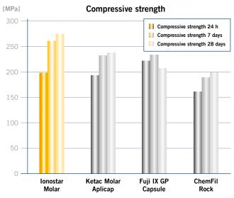
The compressive strength of glass ionomers increases over the course of the retention time, as the material continues to mature and becomes firmer in the process.
